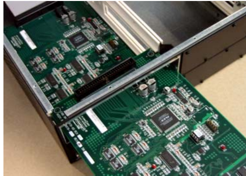
Placing the edge of the card into the guide rails
