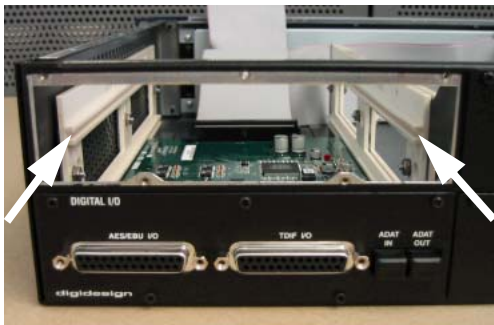
Example of an empty bay. Note guide rails along the inside edge
