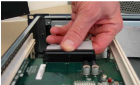
Pressing the 50-pin cable connector into the card
