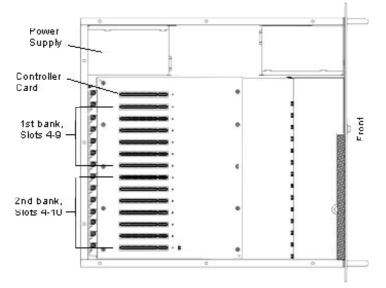
These chassis have slots that are numbered sequentially, right-to-left from the front, in two banks (4-9 and 4-10). Install the controller card in the controller card slot of the expansion chassis (the slot closest to the power supply). This controller card resembles a PCI card.
